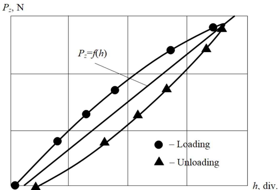
Fig. 4. Calibration graph  $P_z = f(h)$
