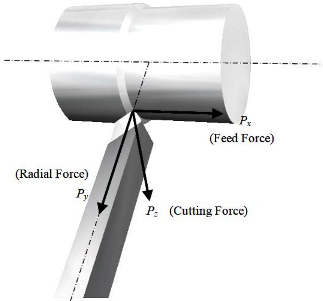
Fig. 1. The forces acting on the cutter
